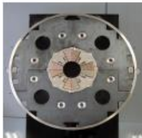
Figure 8.18: (Left) Cross-section of the MQXA low-β quadrupole. (Right) MQXA quadrupole ready for tests in the vertical cryostat in K11K.
